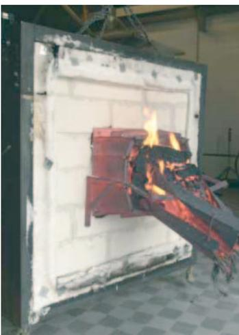
These pictures show the firestopping quality of the Actifoam® rubber. Even with the firestop placed at the exposed side, a two hour fire exposure is possible.
